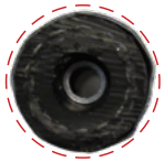
Optimal crimping result obtained with TNT8
