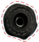
Irregular crimping obtained with other machines not supplied by O+P srl
