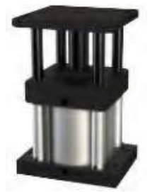
Lifter 4 Post, Ex: 5" bore, 4" stroke, main rod 1.75" dia and the 4 post at 1" dia. The post are guarded by thin wall tubing.
