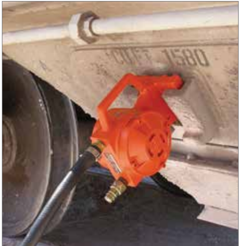
The CCW-5000 unit shown here fits the standard rail car female wedge bracket for easy unloading of a rail road hopper car.
