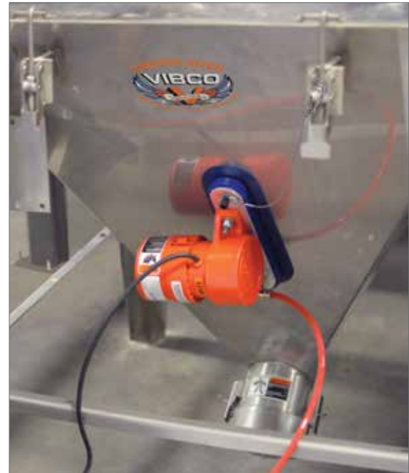
SPR unit (page 40-41) with a Stik-It™ portable vacuum mount does an effective and clean job in keeping the contents of this hopper moving.
