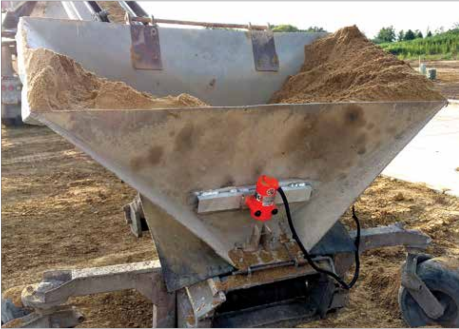
A hopper of sand flows seamlessly onto a conveyor belt with a shake from a US-450 vibrator (see page 46-47). Vibco recommends you follow their manuals (which are put into the box with each order) for proper mounting or consult the factory and use our VVV, Virtual Van Visit™, and mount it right!
