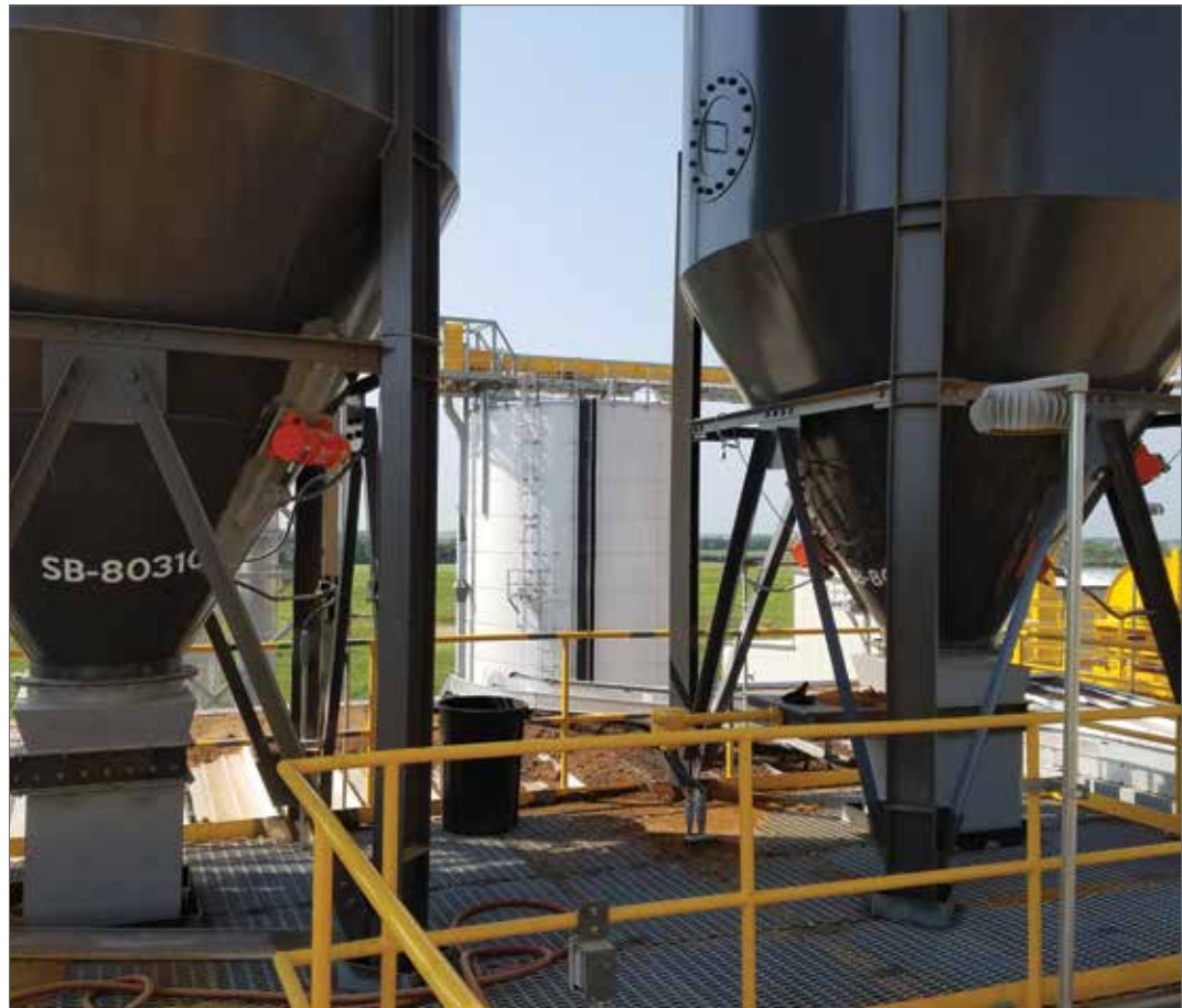
Several Model 2PX explosion proof units (page 52) are used on these twin surge bins.
