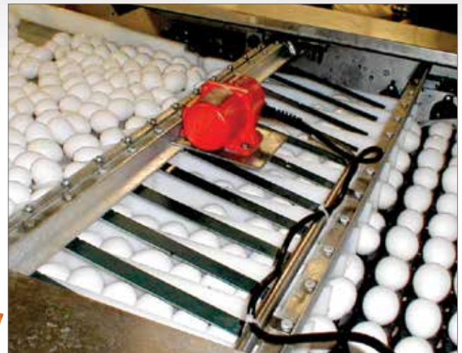
Above: SCR Units are ideal for bins, chutes, packaging, screening, and test tables in rugged conditions, however a Model SCR-60 can also be used with a force and frequency gentle enough to separate egg sizes without scrambling them.
