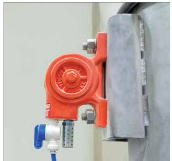
The V-190 shown with optional muffler for noise reduction. A base plate is mounted under the channel for greater efficiency.
