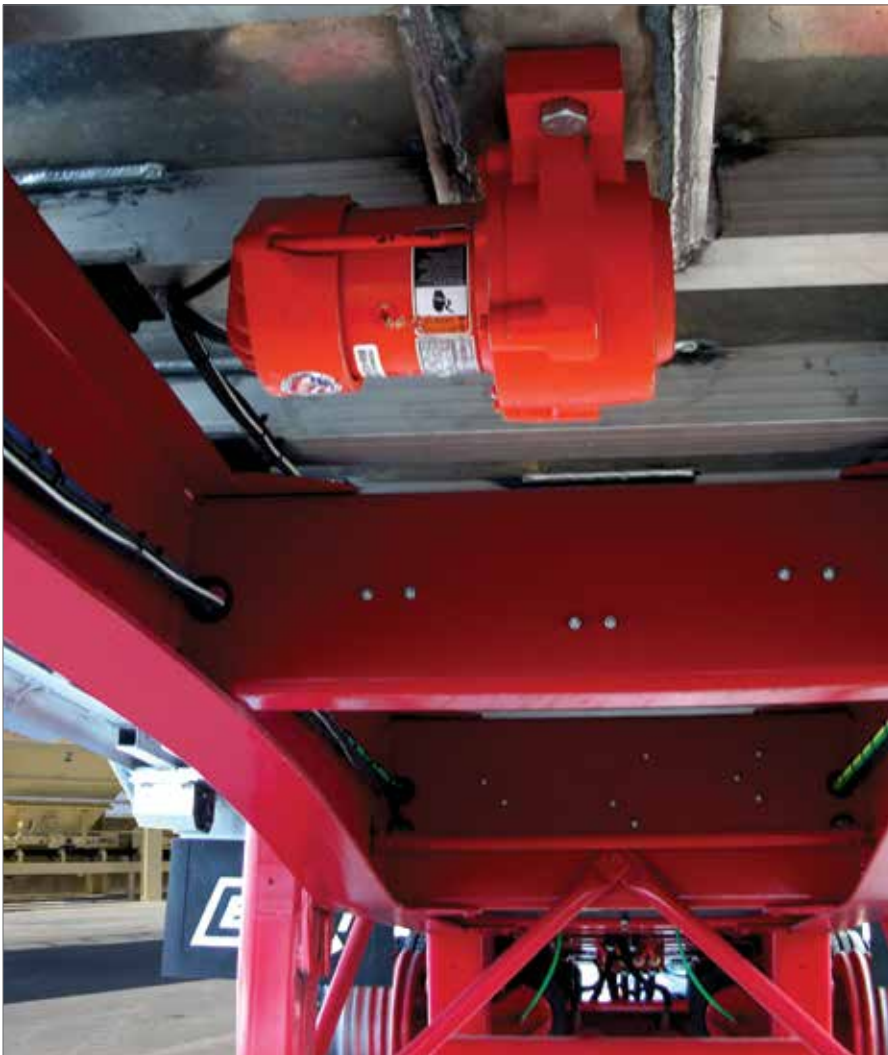
Above: A Big Bertha is used on an excavator to pull large stones and vegetation from a job site while leaving the soil in place (see page 48-49). Below: VIBCO's DC-3500, Big Bertha fits securely beneath the dump body of any truck and comes with all the electrical connections that are needed to install and operate efficiently.
