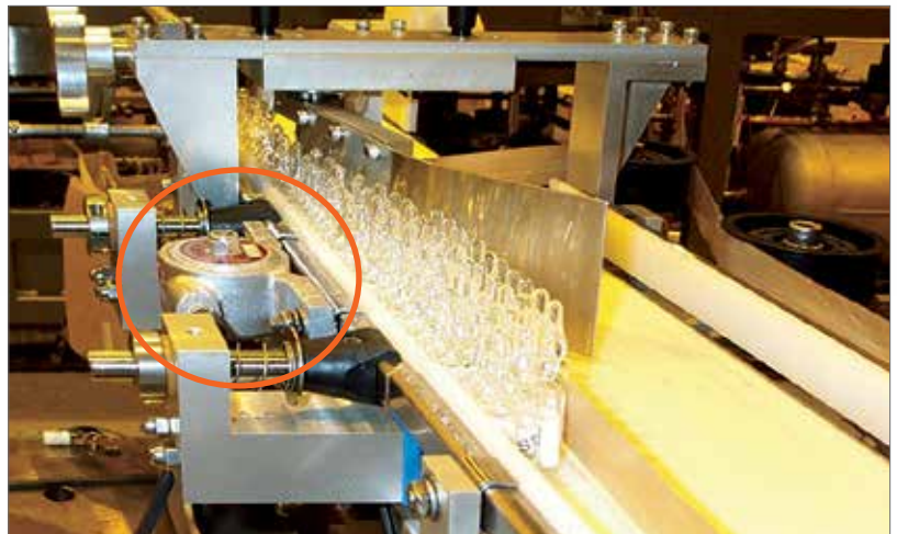
VIBCO's Model VS Turbine Vibrator works equally well on hopper applications (above left) or in conveying delicate glass vaccine bottles as the VS-100 silent Turbine is doing (above) without breakage or getting stuck.
