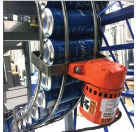
Above: A Model SPR vibrator keeps cans moving, jam-free in this bottling plant.
