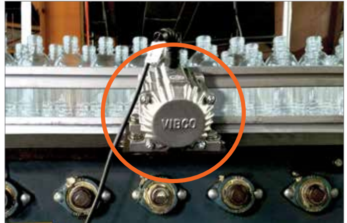
Above: A Model SPWT keeps bottles moving without obstruction on this conveyor. Contact VIBCO for optimal mounting in your specific problem areas.
