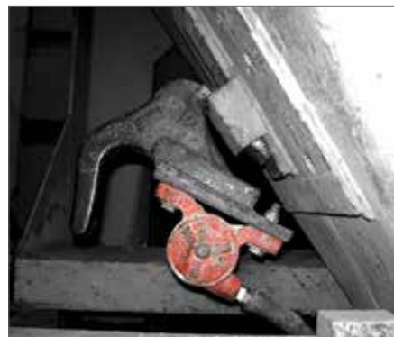
UWF-1 Female Bracket allows multiple hoppers to use one vibrator as needed.
