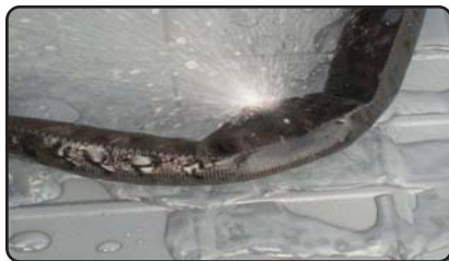
Actual picture of pin hole burst dispersion pattern at 4,000 P.S.I.
