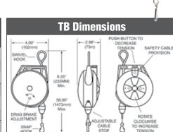
**TBL 15** 10 - 15 4.5 - 6.82.4 10 4.5 YES **TBL 23** 16 - 23 7.2 - 10.42.4 10 4.5 YES \*Cable lengths listed are "active" or "working" cable. Maximum temperature 150 °F (65 °C). \*\*May be adjusted to balance through 6-18 in (152-457 mm) range
