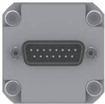
TOP VIEW OF THE REGULATOR CONNECTOR
