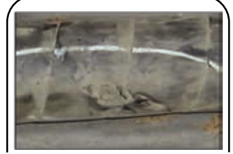
Hole in hose cover that exposes reinforcement
