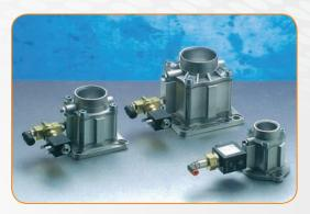
FEC Series - Filters and filtering elements for microfiltration of oils and coolant fluids. Manufactured with high efficiency filter medias, with a filtration rate down to 5 micron, to retain micropollutants. Particularly suitable for diesinking and wire spark erosion machines, machine tools lubrication and cooling systems, grinding procedures etc.
