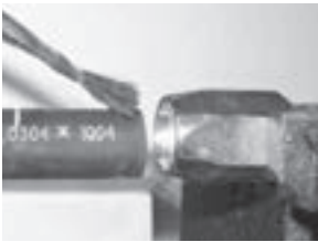
Apply lubricant to hose cover.
