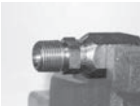
Stem properly seated against socket.
